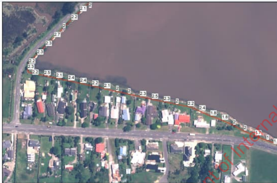
Figure 3.5: Design heights for a future climate 100-year ARI event with RCP6 as proposed within the BBC (Lower Orowaiti) – number labels are height of embankment along its alignment in metres
