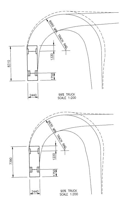
Figure 7.2C - Vehicle tracking curves - bus
